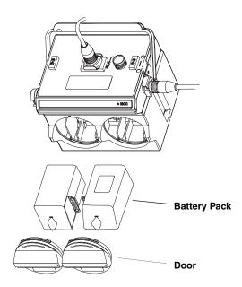
Figure 5-5 Illustration of Battery Packs
